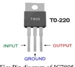
Fig; Pin diagram of IC7805
