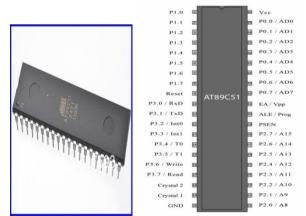
Fig; AT89C51 IC Fig; Pin Description
